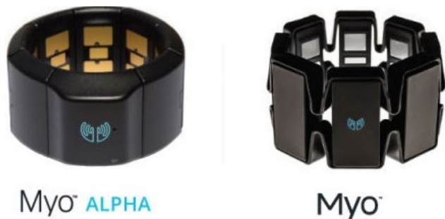
Figure 3. The current form of the Myo (right) is substantially lighter and also more sensitive to bioelectric signals, having moved to medical-grade stainless steel sensors instead of copper-based capacitive PCB sensors. (Image courtesy of Bashny.Net)
